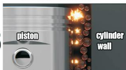
Damage of mineral oil film to cylinder and piston
